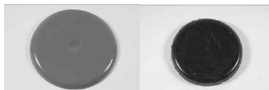
Figure 2. Recycled polymers: recovered: virgin = 1:1 mixture (left), 9:1 mixture (right).
